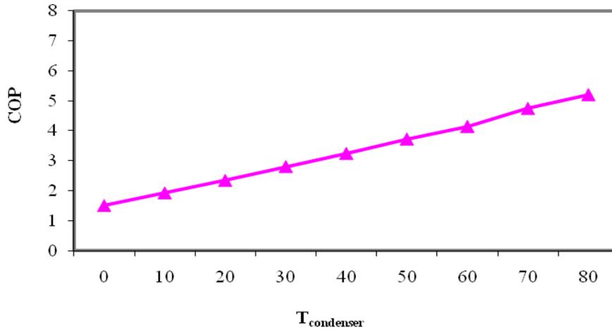
Figure 7. Heat pump performance vs condensation temperature.
