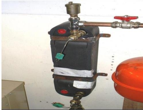
Figure 14. Shows the heat exchanger.
