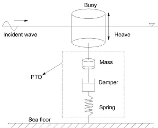
Fig. 3: Schematic display of Heaving point absorber WEC model [8].
