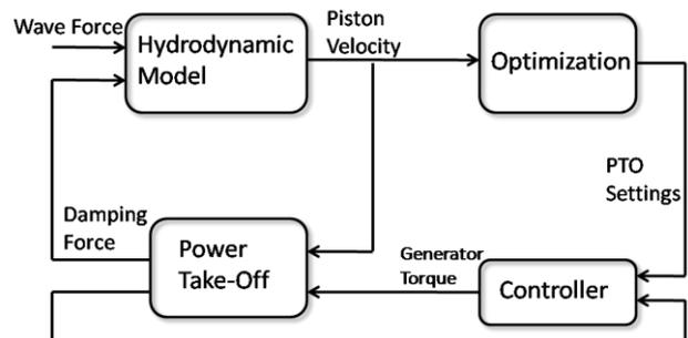
Fig. 10: Representative model of a wave energy converter [13]
