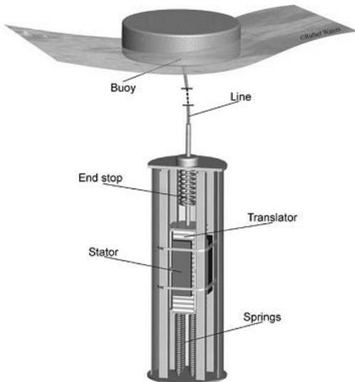
Fig. 2 Heaving buoy with liner electrical generator [6]
