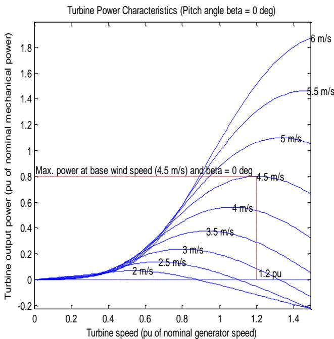
Fig. 9 Wind turbine mechanical output power
