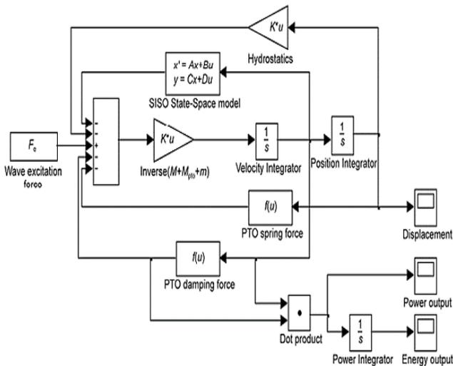
Fig. 11 Simulink model of wave energy converter in time domain (TD) method
