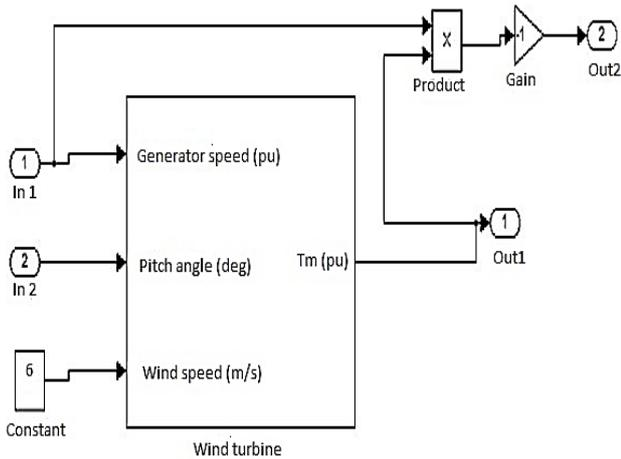
Fig. 8 Simulink model of wind turbine
