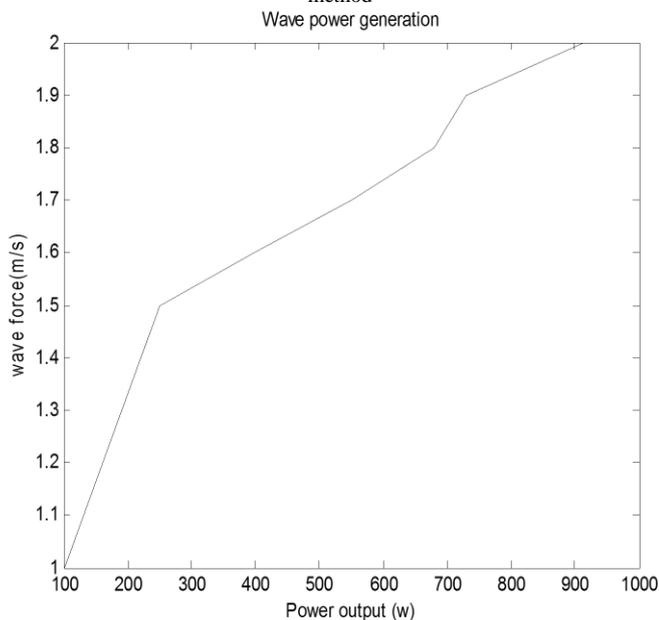
Fig. 12 Wave force excitation versus power output
