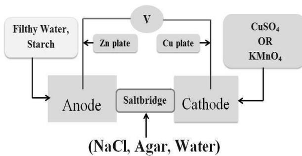
Figure 2. A substitute model of MFC
