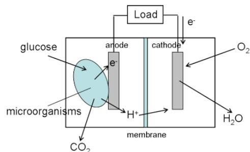
Figure 1. MFC mechanism
