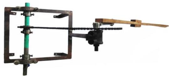
Fig. 3. Structure of Vertical Movement Ocean Wave Generator
