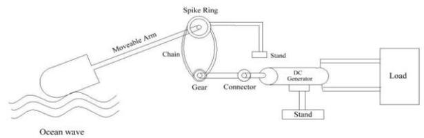
Fig. 2. Design of Vertical Movement Ocean Wave Generator
