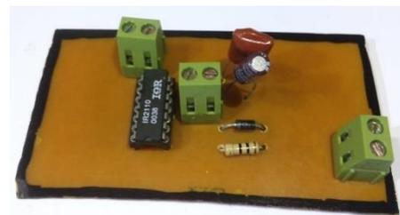
Fig. 19. Gate driver circuit
