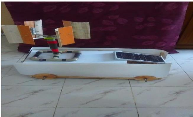
Fig 11: Prototype of green bus model side view
