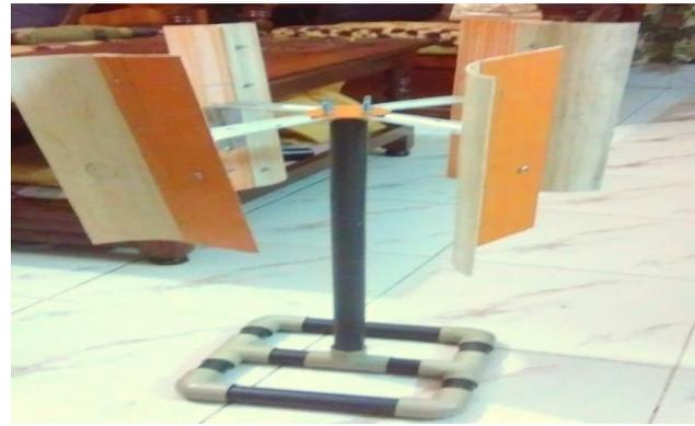
Fig 7: Vertical axis wind turbine made by pvc materials .
