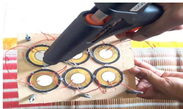
Fig 9: Attaching piezoelectric sensors on hard board
