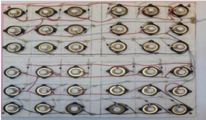
Fig. 4. Physical implementation of 36 piezoelectric sensors
