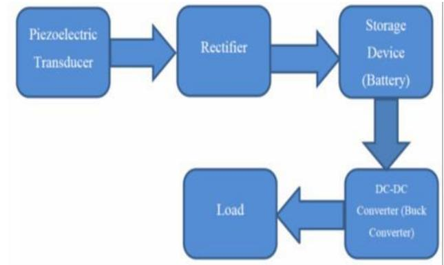
Fig. 1. Block diagram of working principles
