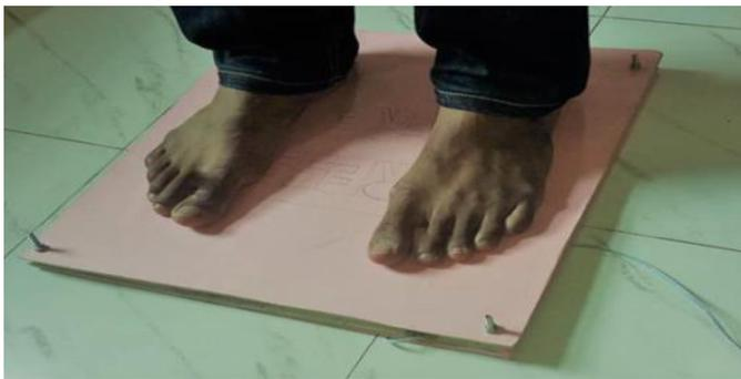
Fig. 5. Mechanical stress was provided on transducer pad
